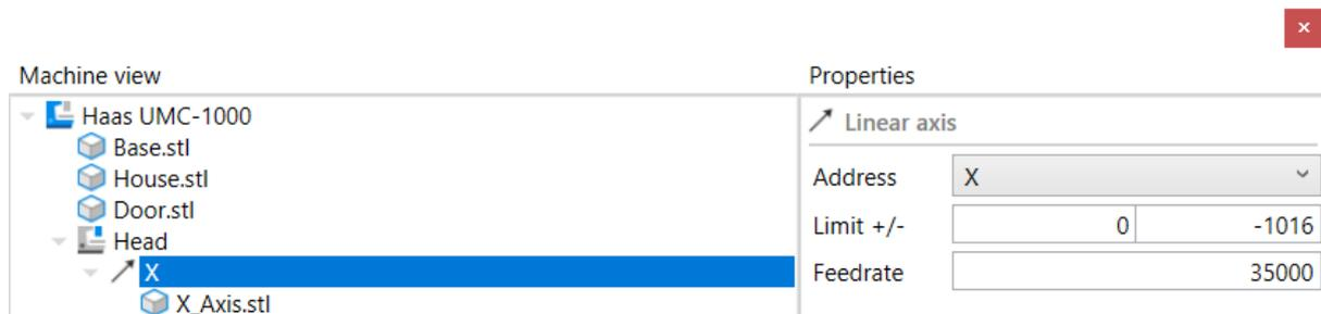
Right-click 'Table' to add a linear axis, a rotary axis or geometry to the table section of the machine.
